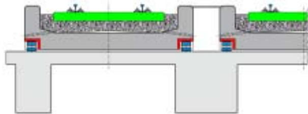
Fig.5 Cross section of the 6 Hz floating trackbed at Puchon Station
