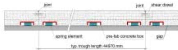
Fig.6 Trough elevation with laterally arranged spring elements
